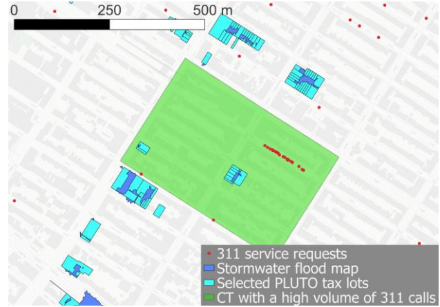
Figure 7: CT where the H&H model might be underestimating the flooding risk (also indicated in red in Figure 6).
